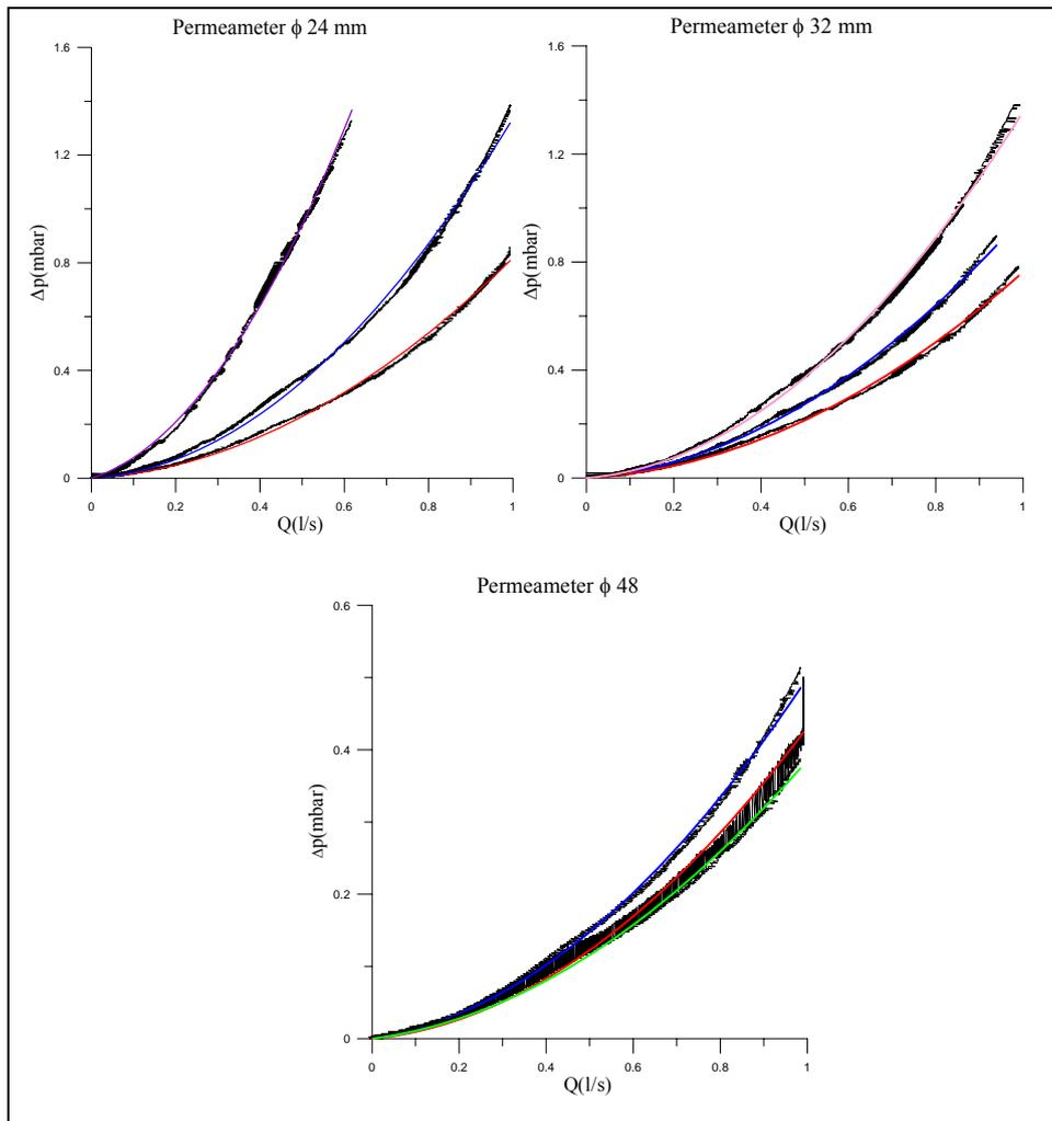
**Figure 3 - Air permeability tests with different permeameter diameters**
