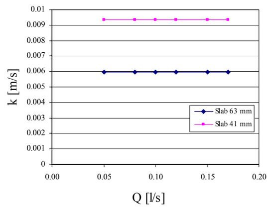
**Figure 6 - Air Permeability k versus discharge for slabs of porous concrete having 41 mm and 63 mm thickness**
