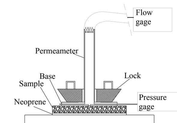
**Figure 2 - Setting procedure with air permeameter**
