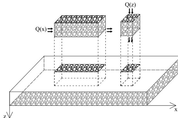
**Figure 1 - One-directional filtration tests on porous asphalt concrete slabs**
