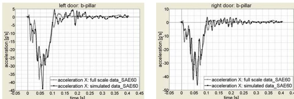
Figure 3: longitudinal acceleration [g's] in 4 different point filtered CFC60
