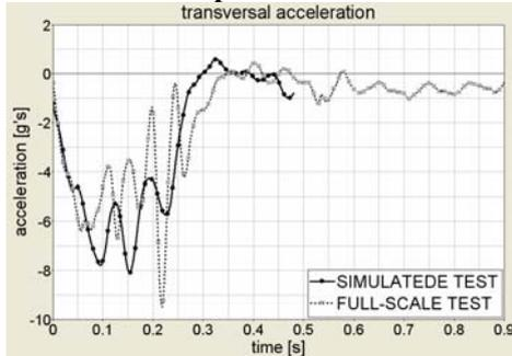
**Figure 4: transversal acceleration [g's] filtered CFC12**
