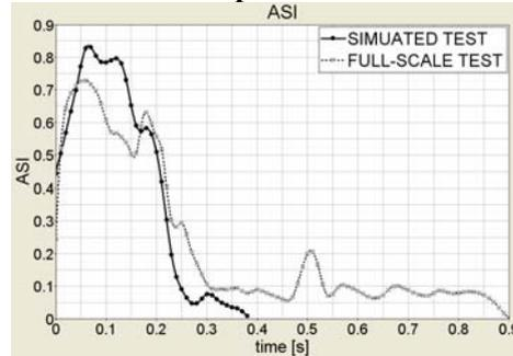
**Figure 5: Acceleration Severity Index (ASI)**
