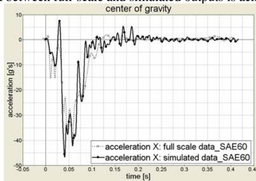
**Figure 2: centre of gravity acceleration [g's] in the longitudinal direction filtered CFC60**
