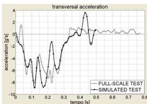
**Figure 7: transversal acceleration [g's] filtered CFC12**
