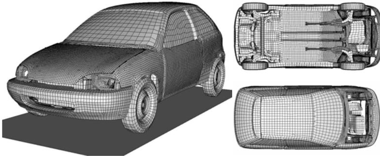
**Figure 1: FE model of the light weight passenger car**
