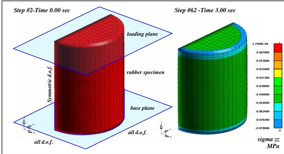
**Figure 6 LS-DYNA3D static model and its final deformation after 3 sec (spec.# 2)**
