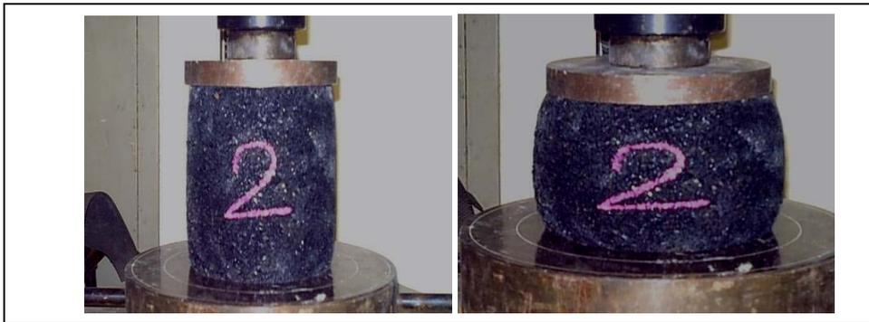
**Figure 2 Static compression test: two instants (4s and 38s) of the same test**
