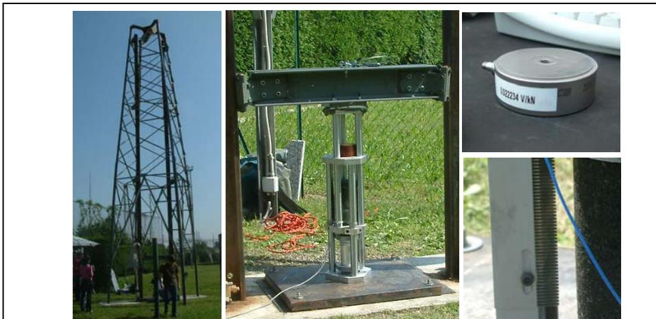
**Figure 4 Dynamic test: tower, loading frame with dart, load cell and encoder for displacement measurements**
