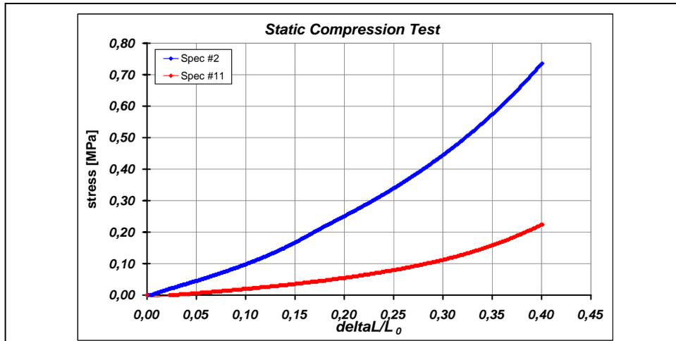
**Figure 3 Static compression test: curves for different densities**
