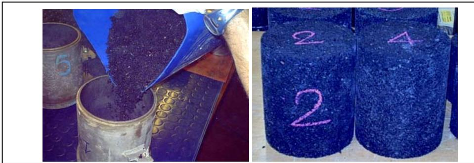
**Figure 1 Laboratory specimens production**
