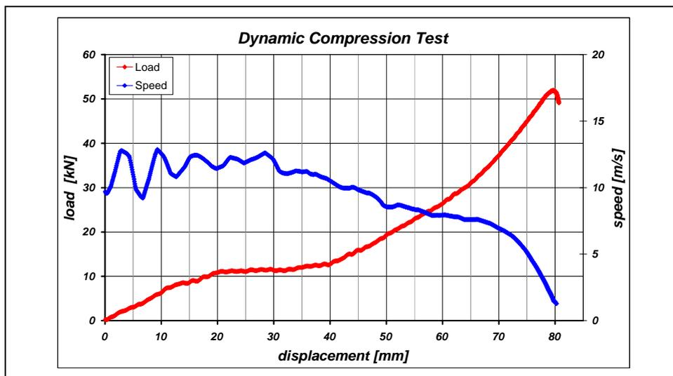
**Figure 5 DCT results: load-displacement curve and speed-displacement curve**
