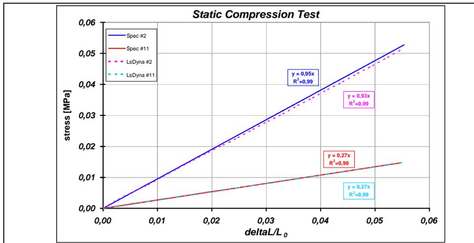
**Figure 7 Laboratory and LS-DYNA3D static curves for different densities**
