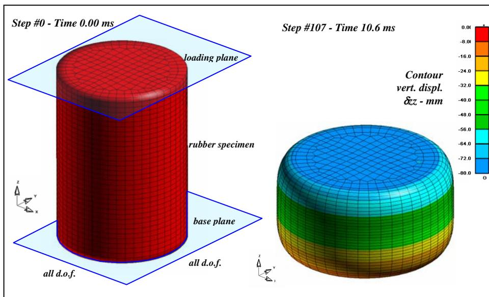
Figure 8 LS-DYNA3D dynamic model and final deformation after 12 ms (spec.#9)
