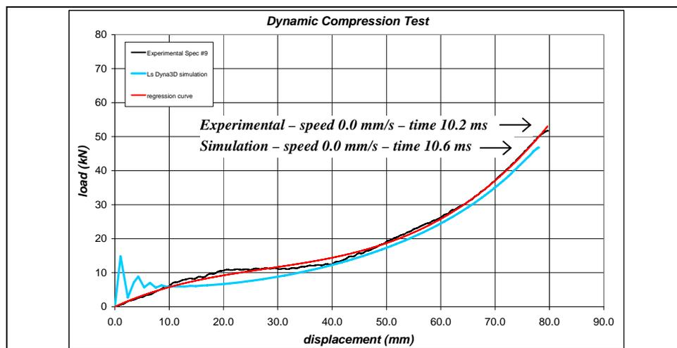
**Figure 9 Laboratory and LS-DYNA3D curves for dynamic tests (spec.#9)**
