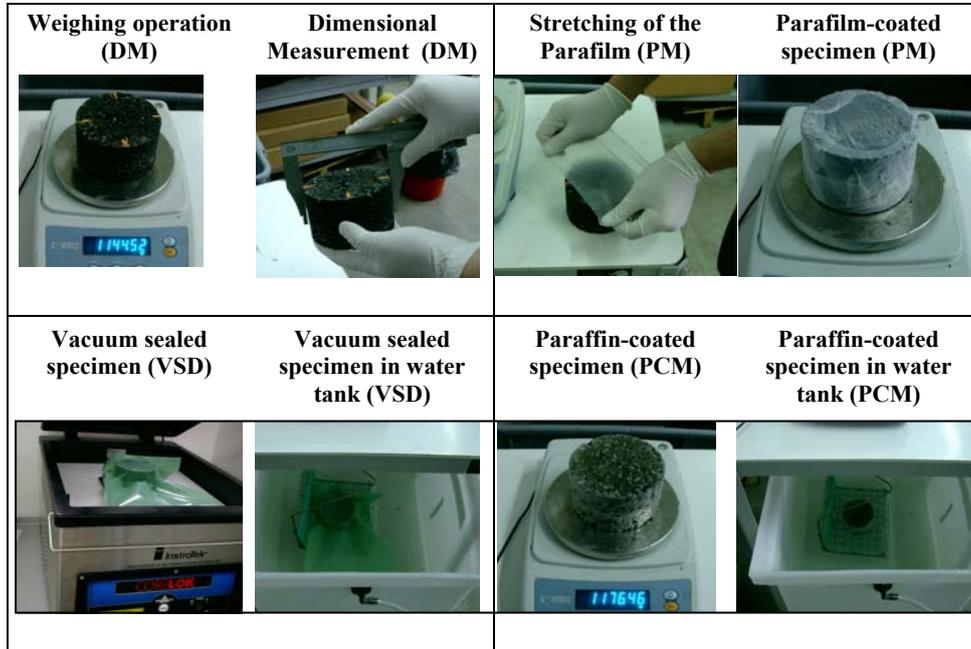
Figure 5 Main Phases for the four procedures
