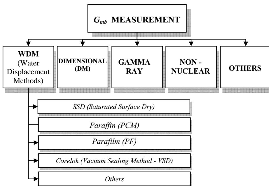
Figure 1 Main Methods for  $G_{mb}$  Measurement
