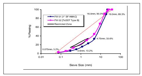
Figure 3 Aggregate Gradations
