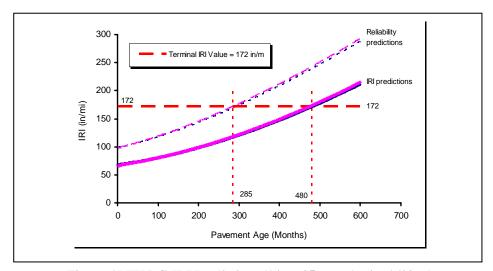
Figure 6 MEPDG IRI Predictions (1 in ≅ 25 mm; 1 mi ≅ 1609 m)
