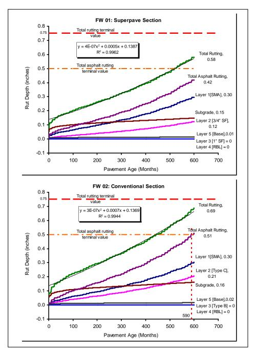
**Figure 5 MEPDG Permanent Deformation and Rutting Predictions** (1 inch ≅ 25 mm; <sup>3</sup>⁄<sub>4</sub>" SF = <sup>3</sup>⁄<sub>4</sub>" SFHMAC [19 mm NMAS]; 1" SF = 1" SFHMAC [25 mm NMAS])
