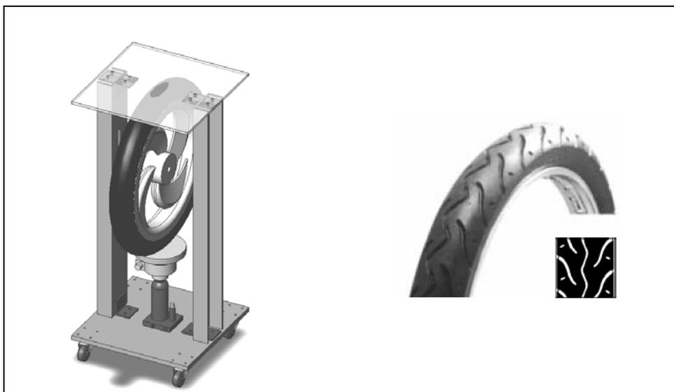
**Figure 1** Tire-plate contact. Left: arrangement of the components for the ultrasonic analysis, Right: tire tread pattern
