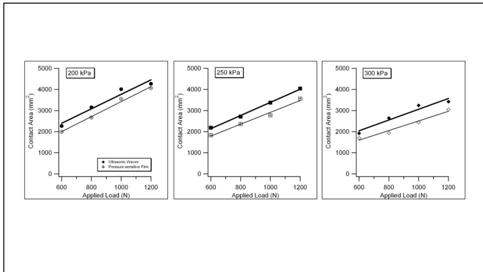
**Figure 5 Comparison between the contact area values obtained from ultrasonic and those from pressure-sensitive film tests**
