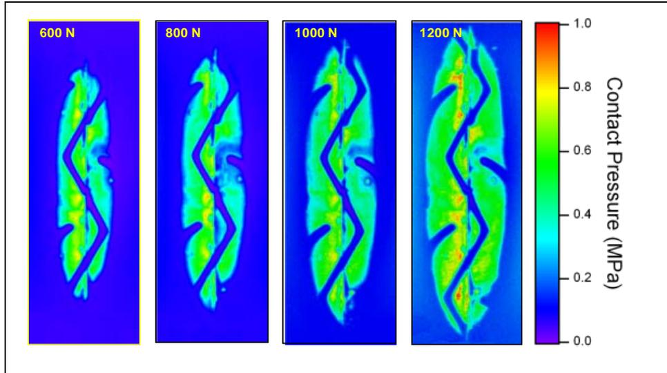
**Figure 3 Ultrasonic maps of contact: evolution of the contact ellipse for increasing applied loads (inflation pressure 250 kPa)**
