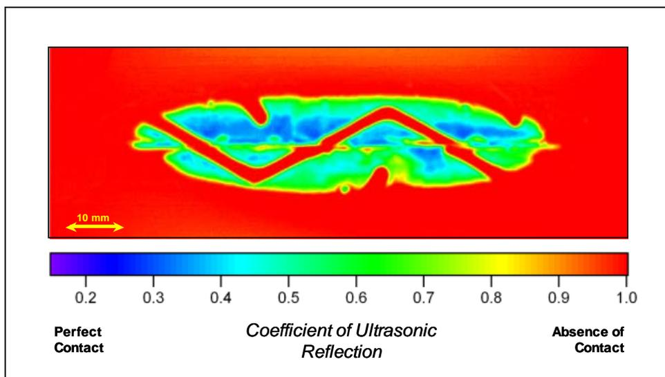
**Figure 2** Graphic processing of ultrasonic reflection data for a tire-plate contact (applied load 600 N, inflation pressure 250 kPa)
