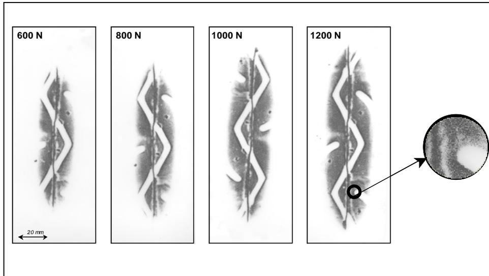
**Figure 4 Evolution of the contact ellipse for increasing applied loads as obtained from the pressure-sensitive film tests (inflation pressure 250 kPa)
