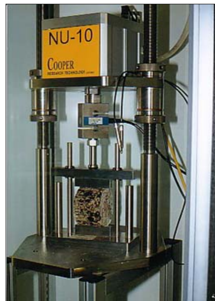
Figure 3: Indirect tensile fatigue set up
