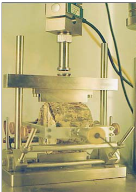
Figure 2: Indirect tensile modulus set up
