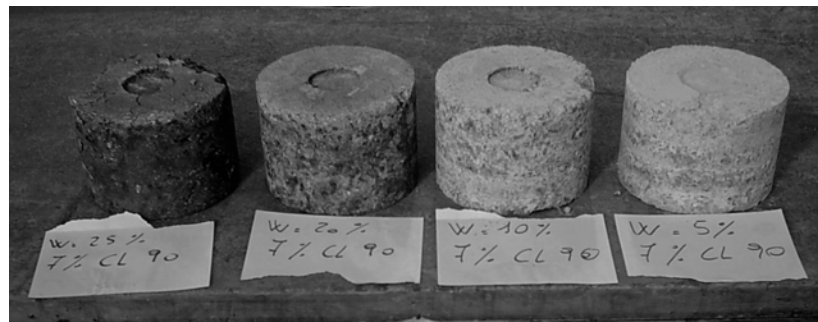
Figure 12: Test pieces made up with different percentages of water
