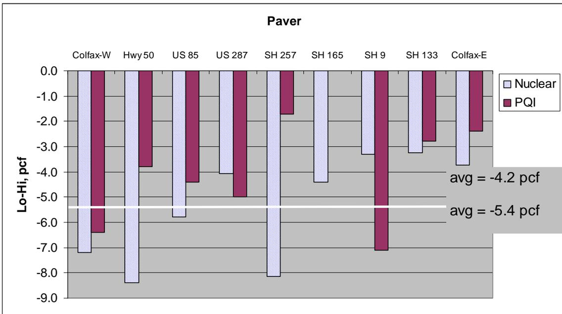
Figure 15- Nuclear and PQI Density Comparison for 'Paver' Data
