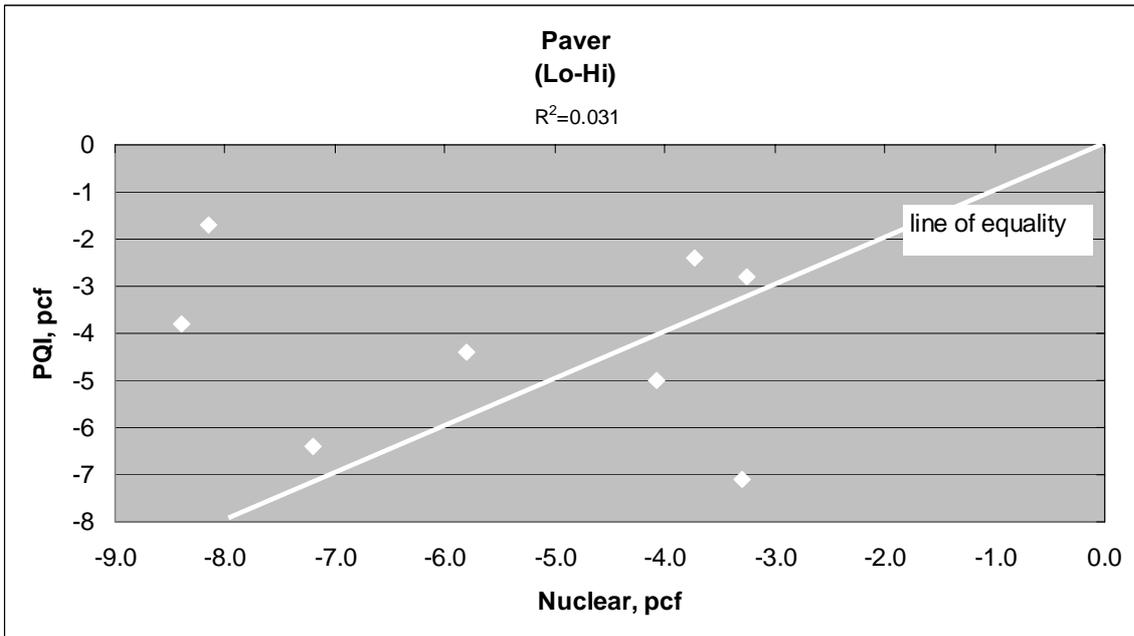
Figure 16 – Regression Analysis of Nuclear and PQI ‘Paver’ Data
