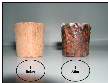
Figure 6: Stopper type 1 before/after compaction (PI)
