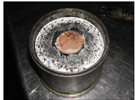
Figure 15: Compacted Marshall specimen and embedded stopper
