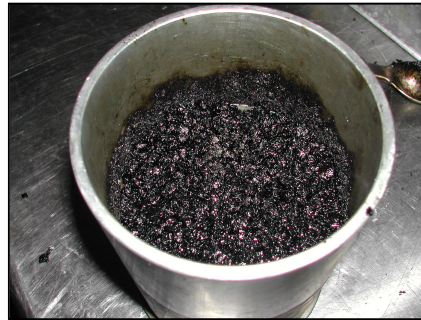
Figure 14: Hot mix asphalt in the Marshall mould
