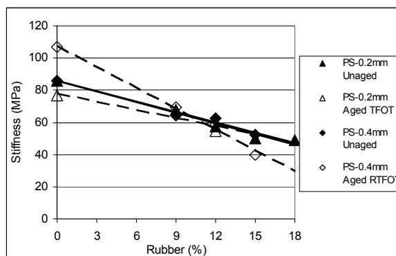
Figure 6: Flexural Creep Stiffness at  $-10^{\circ}\text{C}$
