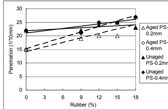
**Figure 3: Penetration test at 4°C**
