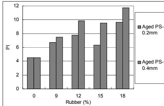
Figure 5: Penetration Index (PI) after aging
