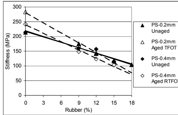
**Figure 7: Flexural Creep Stiffness at -15°C**
