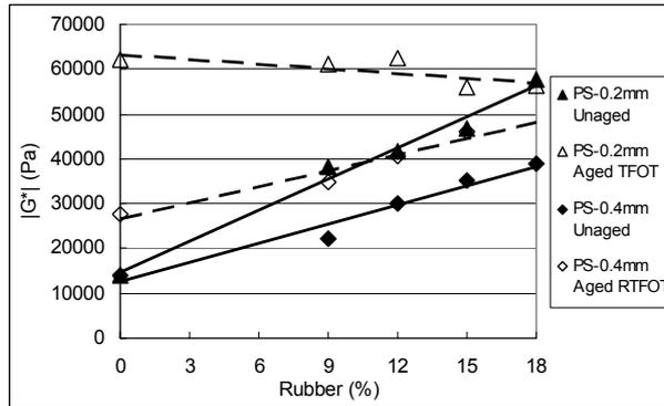
Figure 10: Complex Shear Modulus ( $|G^*|$ ) at 45°C
