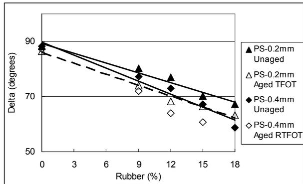
Figure 13: Phase angle ( $\delta$ ) at 65°C
