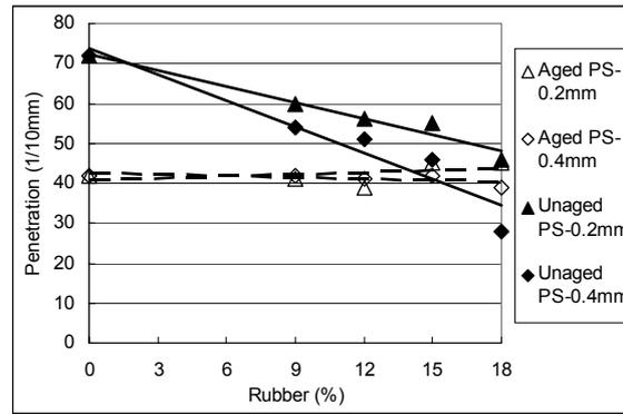
**Figure 2: Penetration test at 25°C**
