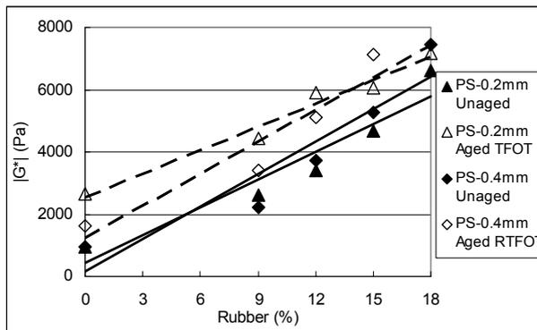
Figure 11: Complex Shear Modulus ( $|G^*|$ ) at 65°C
