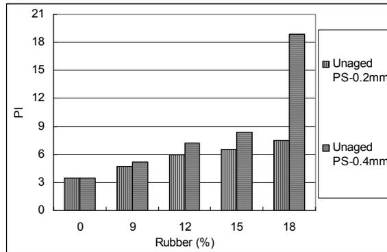
Figure 4: Penetration Index (PI) before oxidation
