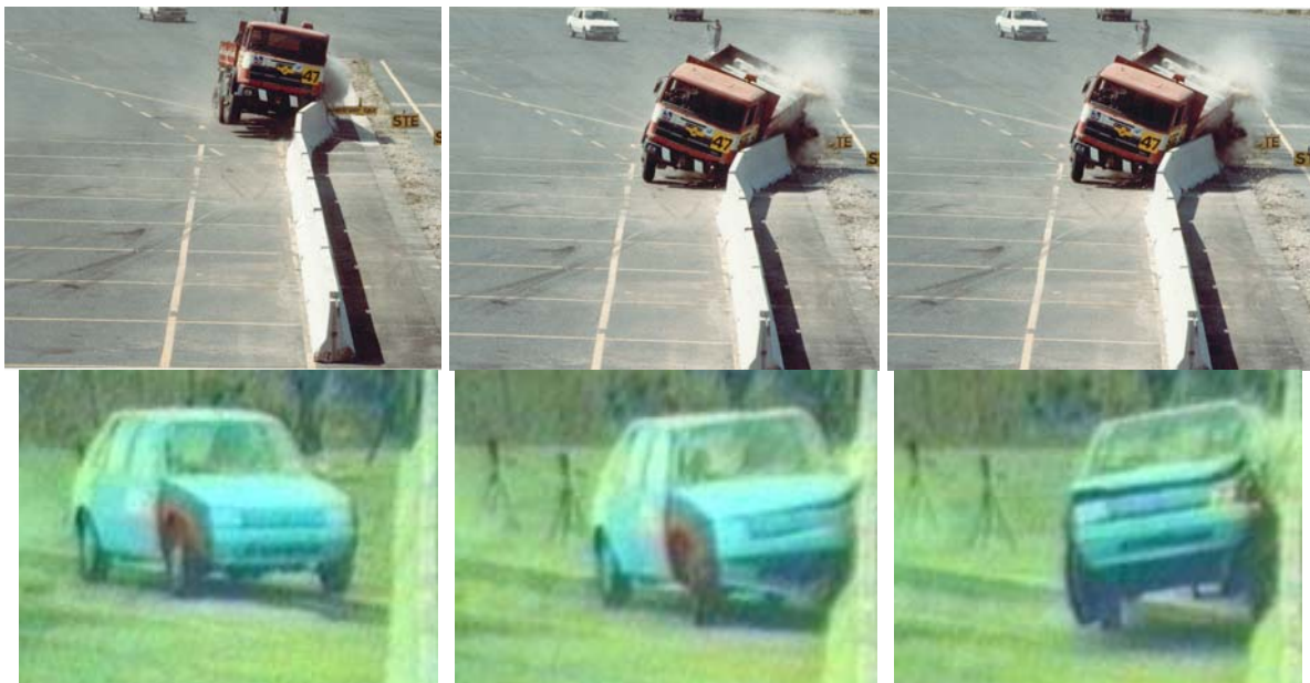
Figure 1 – Example of laboratory crash test, performed for the homologation of safety barriers
