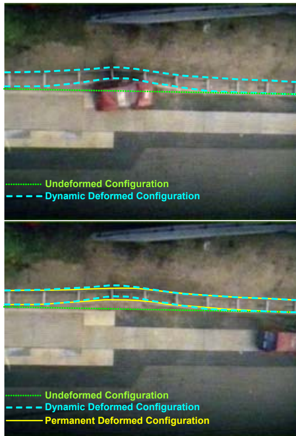
Figure 3 – The impact phenomenon shown with the evolution of the device deformations
