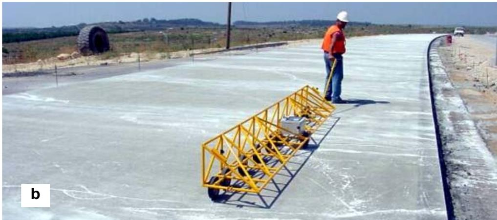
**Figure 1. The German Planograph of the Riedhofer Messtechnik V. 0.12 type: (a) a side elevation view; (b) as utilized on Route 3**
