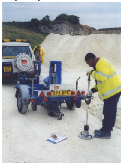
Figure 1 Falling Weight Deflectometer (FWD) and Light Weight Deflectometer (LWD) Tests on a foundation
