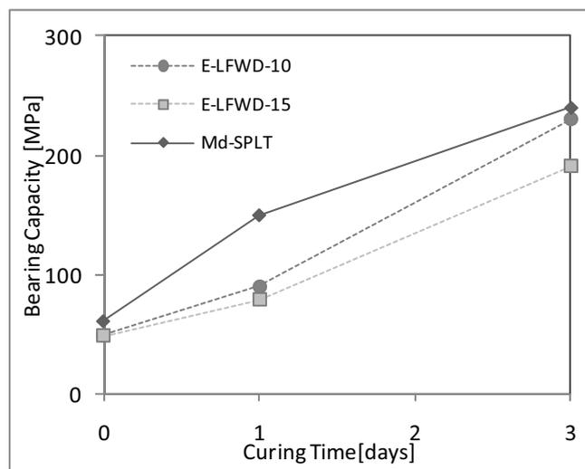
Figure 7. In situ mechanical test results on CTB
