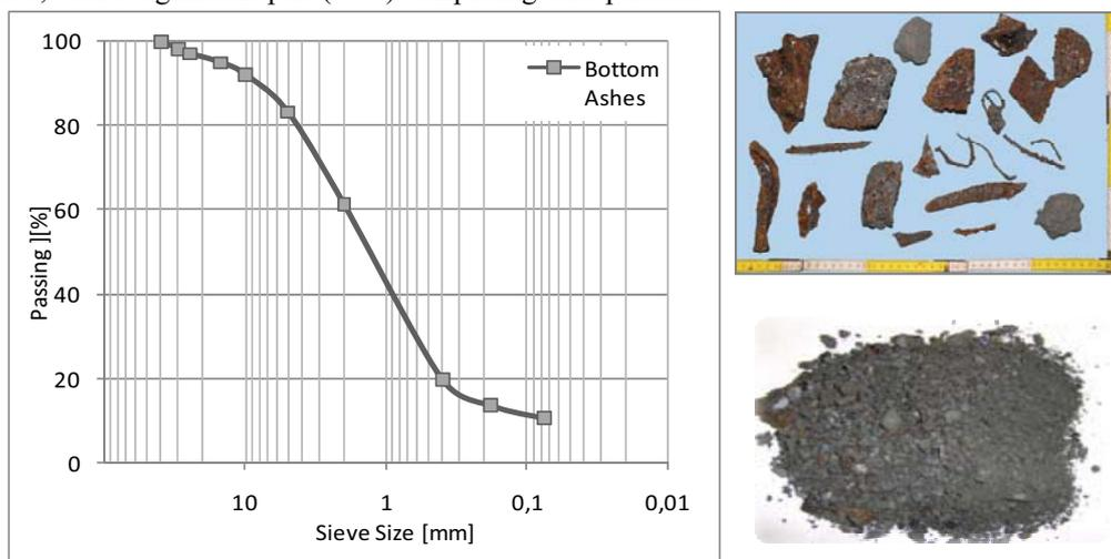
Figure 3. Particle size distribution of SBAs, removed pieces, SBAs used in the tests.
