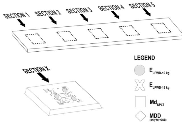
Figure 2. Test methods used to measure the materials' field performance
