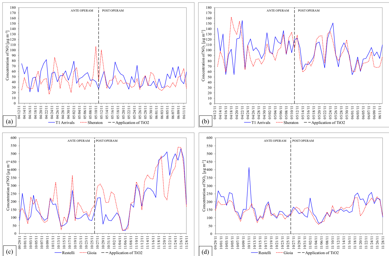
Figure 4: Maximum daily concentration of NO and NO 2 : a), b) Malpensa Airport c), d) Milan.
