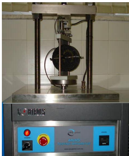
Fig. 1 (a) Fatigue test equipment; (b) Fatigue curves
