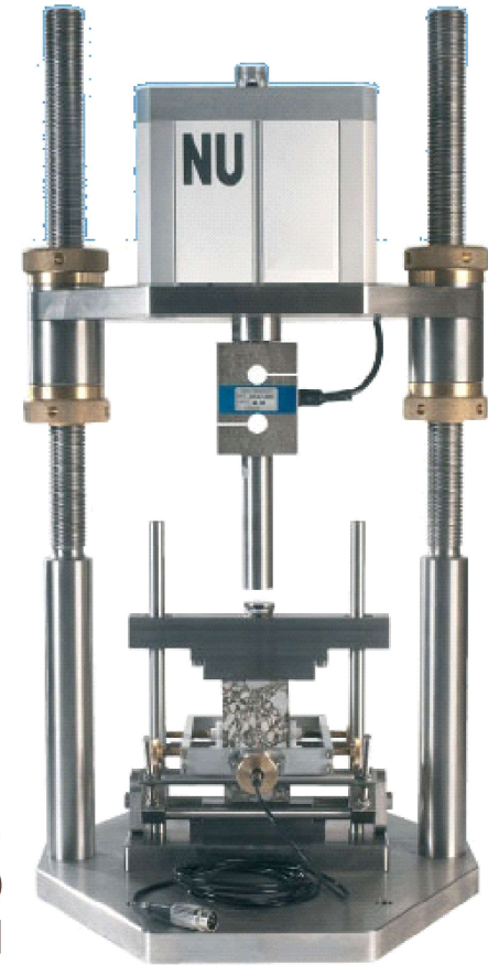
Stiffness Modulus test (EN 12697-26) Performance based
