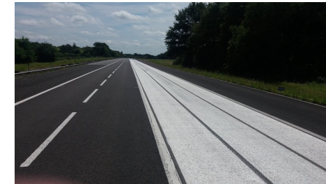
Test track dedicated to skid resistance issues, Ifsttar-Nantes
