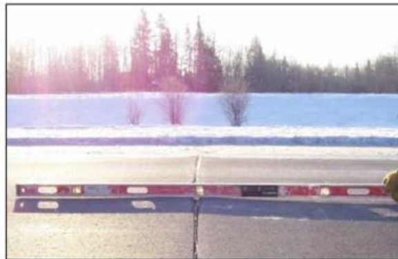
Manual measurement of a tented crack
