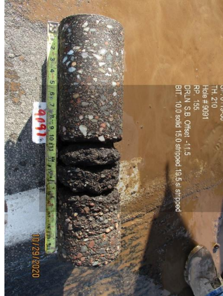
Stripping at the bottom layer of Full Depth AC pavement
