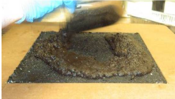
Figure 3.16: Preparation of slurry surfacings slabs
