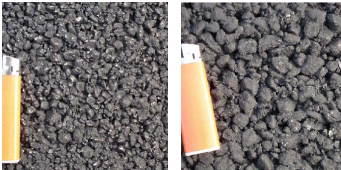
Figure 1.17: Different porous asphalts surface textures
