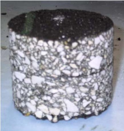
**Figure 3.4: Typical cylindrical specimen for ASTRA**
