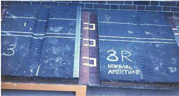
Figure 1.6: Comparison between reinforced and unreinforced slab (Brown et al., 1985).
