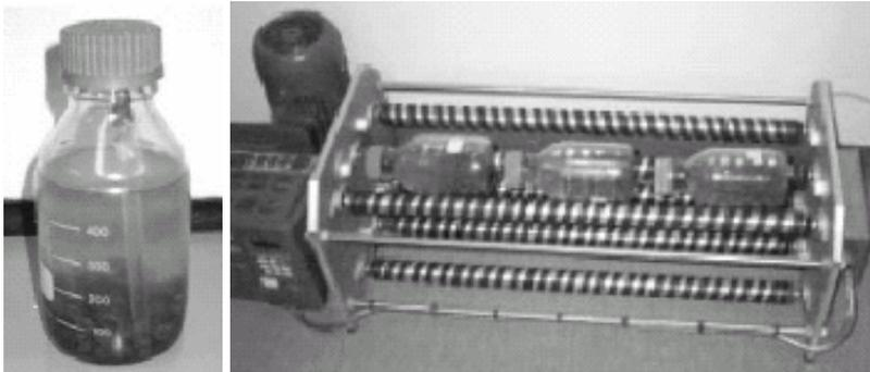
**Figure 6.1: Test bottle and bottle rolling machine for EN 12697-11**
