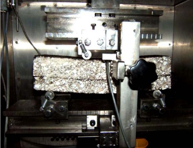
**Figure 4.15: Four point bending test device**
