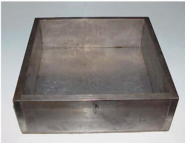
**Figure 4.2: Roller Compactor mould**
