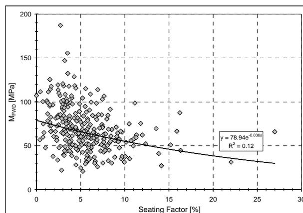
**Figure 5. Surface modulus from FWD testing versus the seating factor for a compacted silty-clay material at the recent airfield project in Israel**
