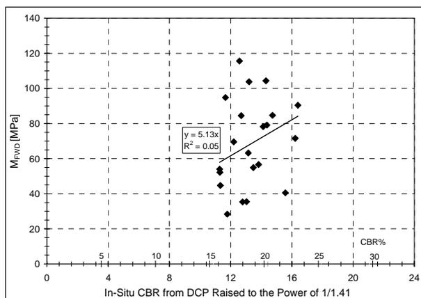
**Figure 1. Surface modulus from FWD testing versus in-situ CBR, as obtained in compacted silty-clay material from the recent airfield project in Israel**
