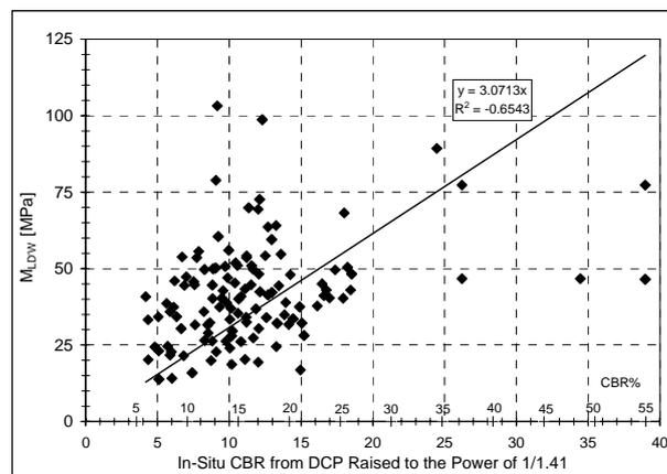
**Figure 2. Surface modulus from LDW testing versus in-situ CBR, as obtained in natural silty-clay material from the recent airfield project in Israel**
