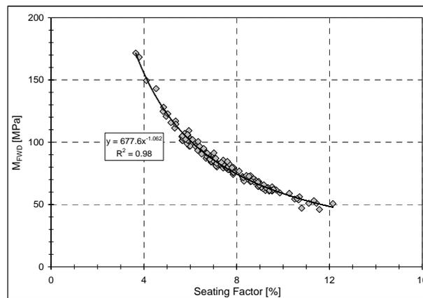
**Figure 4. Surface modulus from FWD testing versus the seating factor for a compacted sandy material at a major road construction project in Israel**
