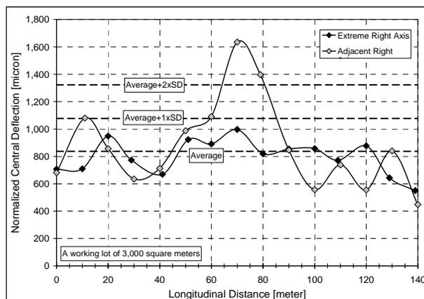
**Figure 6. FWD measurements of central deflection (normalized to 22 kN), made along a working lot of compacted silty-clay material**
