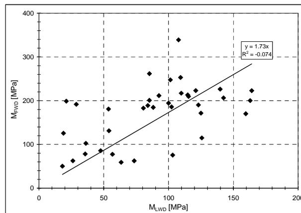
**Figure 3. Surface modulus from FWD testing versus surface modulus from LDW testing, as obtained in compacted chalky-marl material in Israel**
