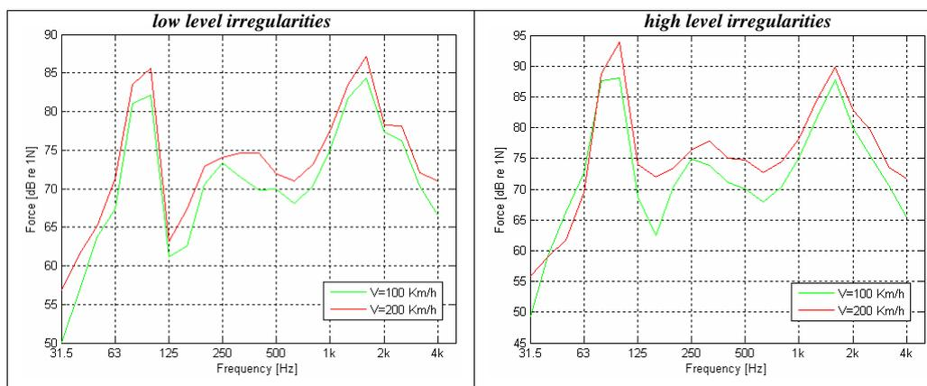
**Fig. 11 - Contact forces response spectrum in 1/3 band of octave of Fig. 10 signals**
