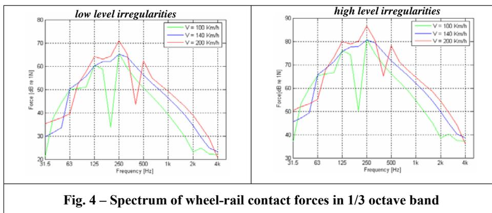
**Fig. 4 – Spectrum of wheel-rail contact forces in 1/3 octave band**
