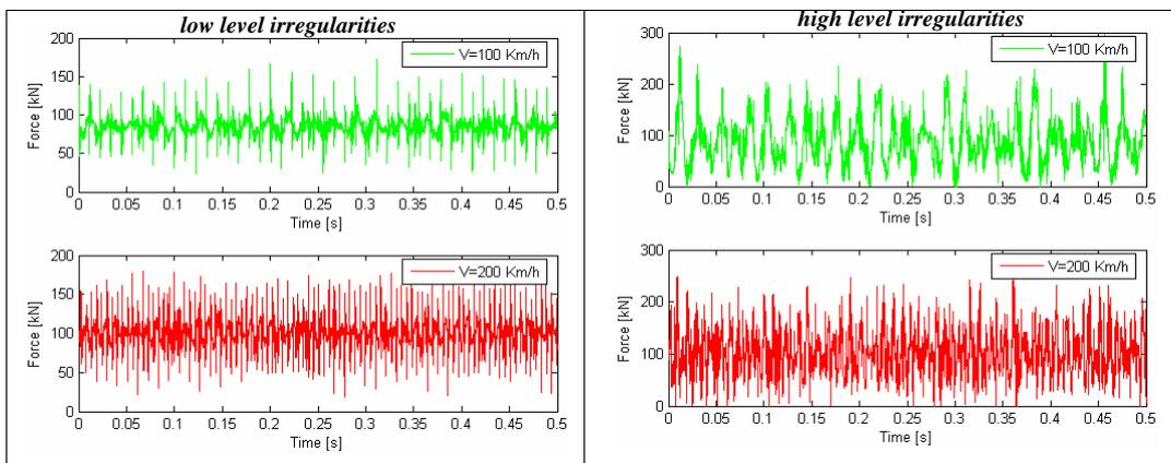
**Fig. 10 - Contact forces induced by low and high level irregularities, at two different speeds**
