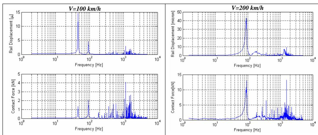
**Fig. 8 - Rail vibrations and contact forces in spectral form, at two different speeds**
