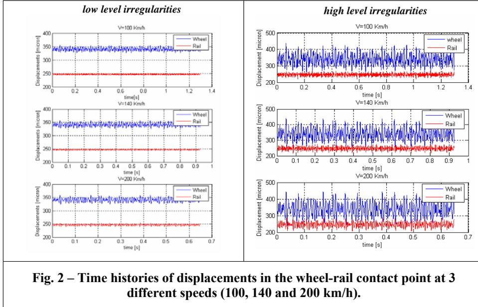
**Fig. 2 – Time histories of displacements in the wheel-rail contact point at 3 different speeds (100, 140 and 200 km/h).**
