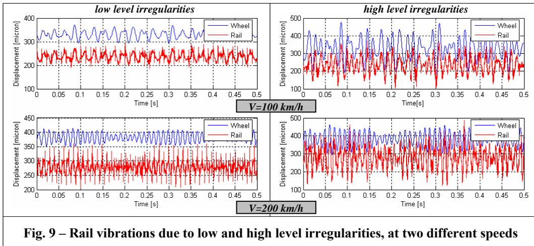
**Fig. 9 – Rail vibrations due to low and high level irregularities, at two different speeds**
