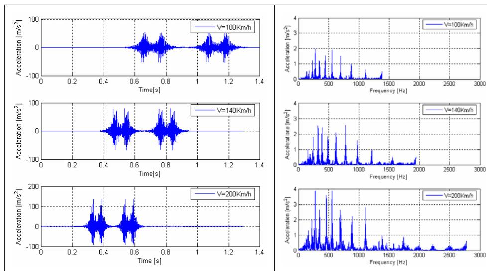
**Fig. 15 – Signals and spectrums of accelerations: 3 speeds, rail node and high-level of irregularity**
