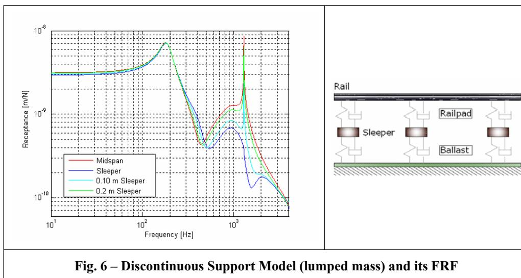
**Fig. 6 – Discontinuous Support Model (lumped mass) and its FRF**
