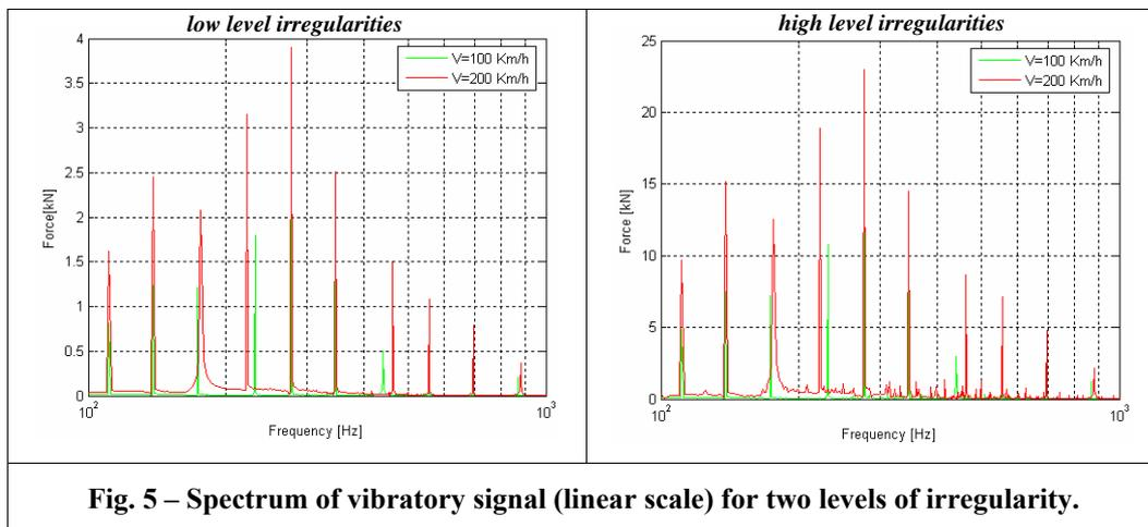
**Fig. 5 – Spectrum of vibratory signal (linear scale) for two levels of irregularity.**
