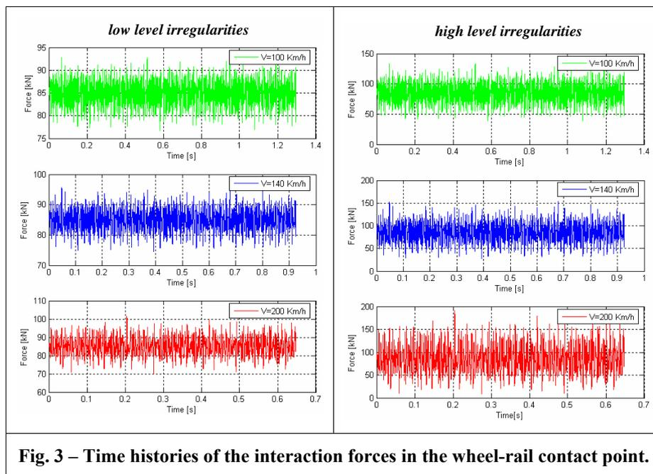
**Fig. 3 – Time histories of the interaction forces in the wheel-rail contact point.**
