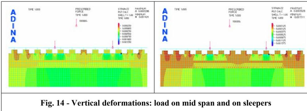
**Fig. 14 - Vertical deformations: load on mid span and on sleepers**
