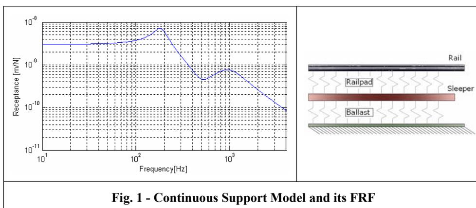
**Fig. 1 - Continuous Support Model and its FRF**
