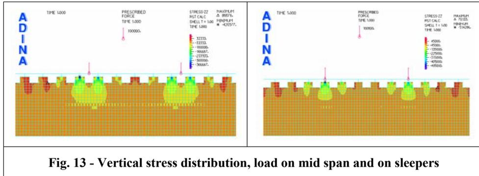
**Fig. 13 - Vertical stress distribution, load on mid span and on sleepers**
