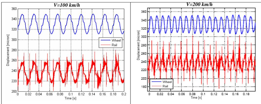
**Fig. 7 - Wheel and rail vibrations in the contact point, only due to parametric excitement, at two different speeds (100 and 200 km/h)**
