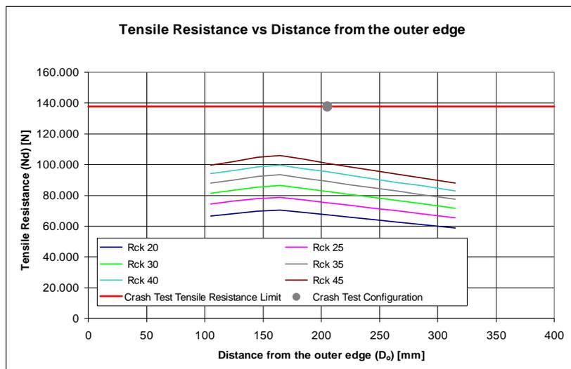
Figure 8 - Influence of Rck and  $D_o$  on tensile resistance (support width=500 mm)
