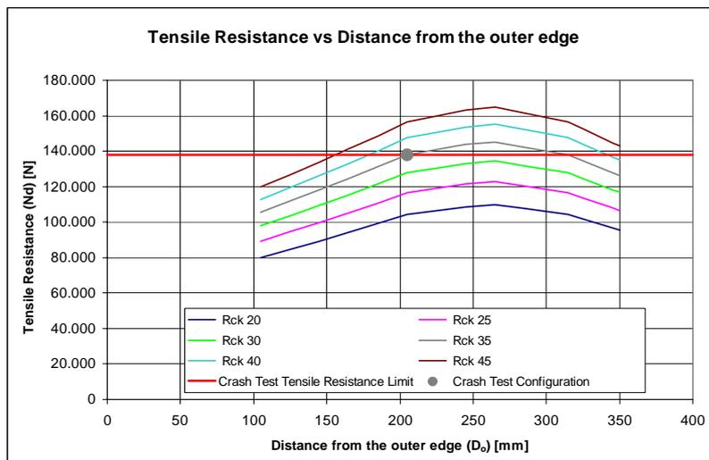
Figure 7 - Influence of  $R_{ck}$  and  $D_o$  on tensile resistance (support width=700 mm)
