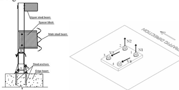
**Figure 1 - Schematization of the actions on the bridge rail anchors**
