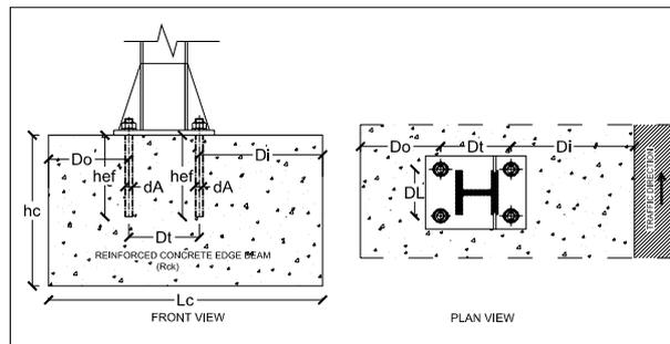
Figure 2 - Geometric description of the anchoring system and concrete support
