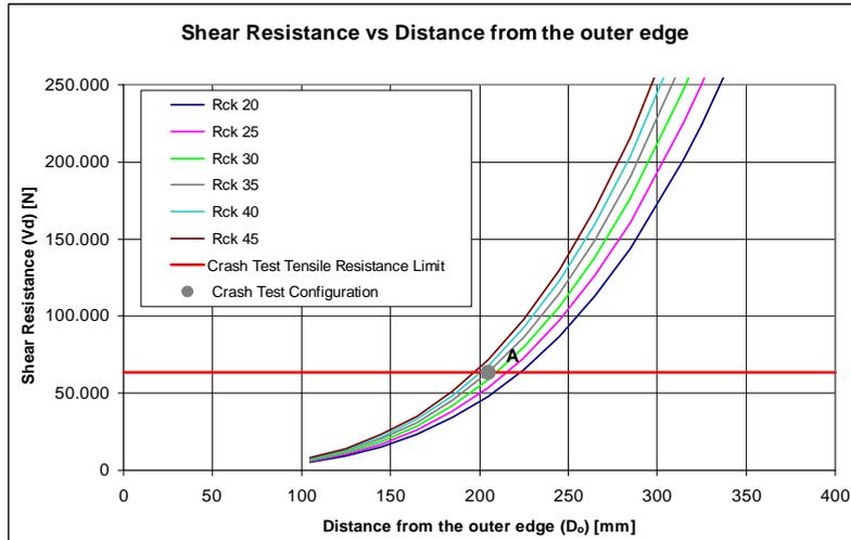
Figure 6 - Influence of  $R_{ck}$  and  $D_o$  on shear resistance
