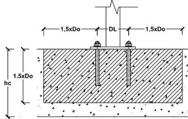
Figure 4 - Definition of the anchors group influence area for shear strength
