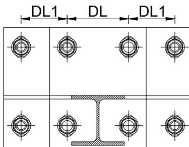
**Figure 10 - Anchoring system with increased number of anchors (from 4 to 8).**
