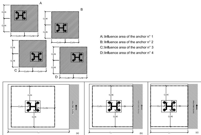
Figure 3 - Definition of the anchors group influence area for tensile strength
