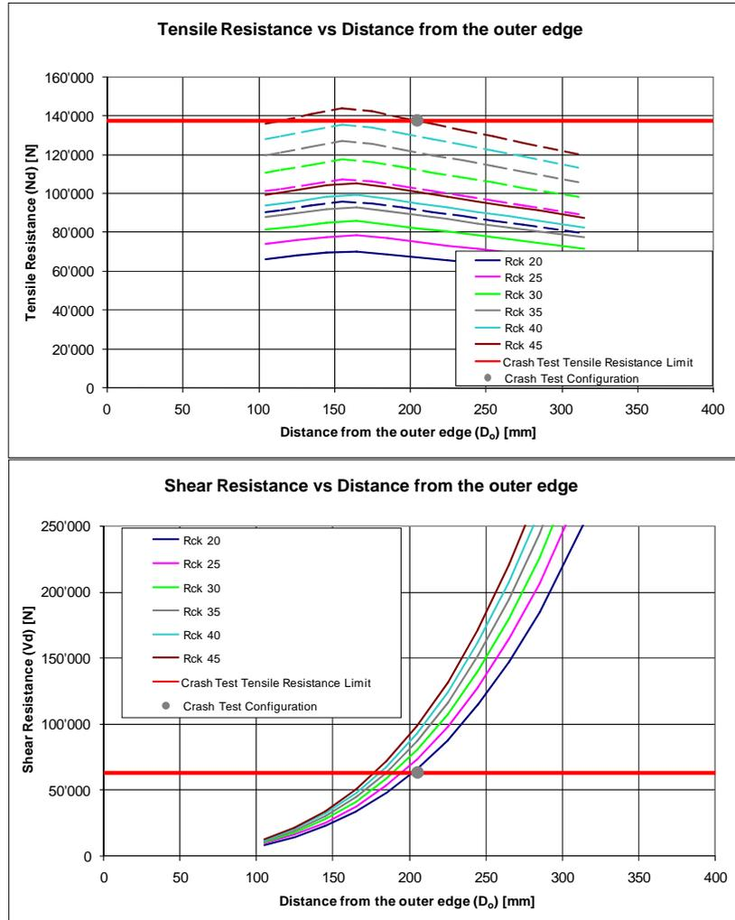
**Figure 11 - Influence of Rck and D<sub>o</sub> on tensile resistance (upper) and shear strength (lower) (support width=500 mm) with 4 anchors (solid lines) and 8 anchors (dashed lines)**
