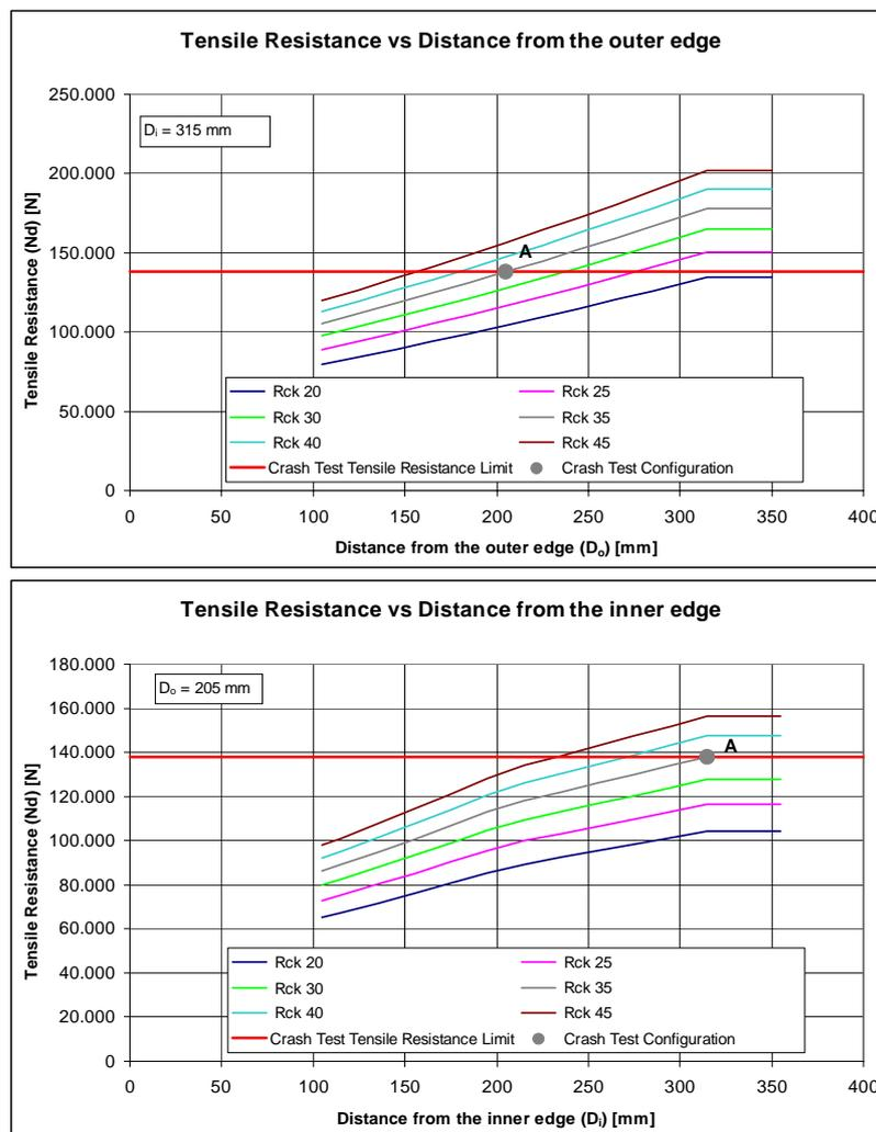
**Figure 5 - Influence of Rck and  $D_o$  (upper) and  $D_i$  (lower) on tensile resistance**
