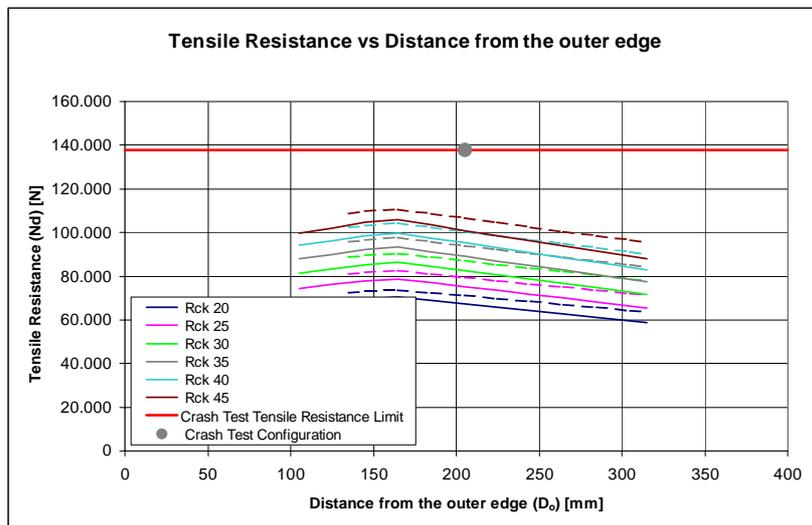
Figure 9 - Influence of Rck and D<sub>o</sub> on tensile resistance (support width=500 mm) with anchor types M24 (solid lines) and M30 (dashed lines).
