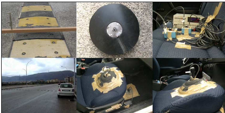
Figure 3 – Irregularity sample and equipment used in field tests [5].
