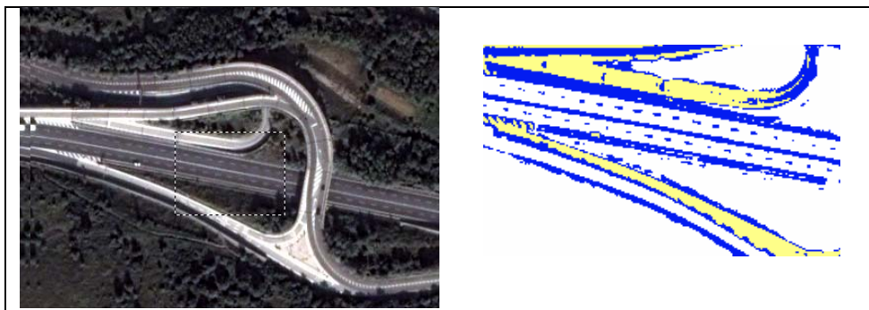
Figure 4 Particular of road signing extraction
