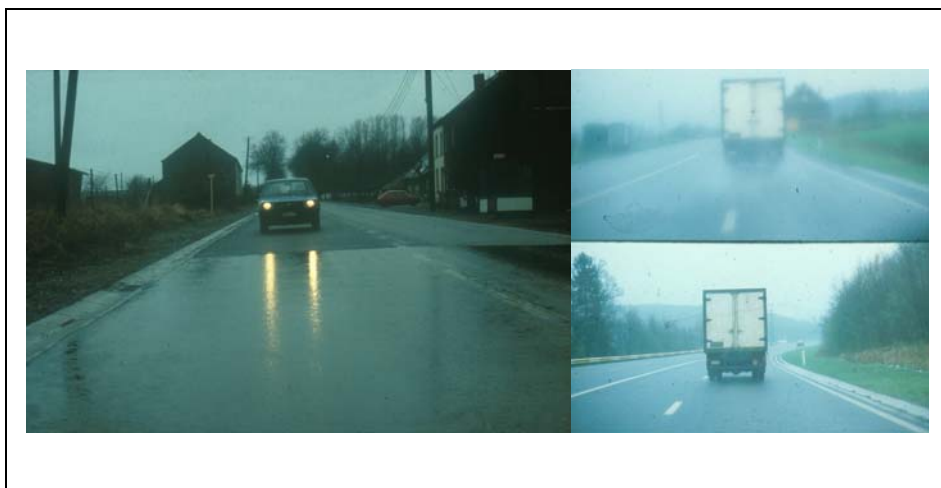
Figure 3 Additional benefits of porous surfaces: less glare and spray in wet conditions
