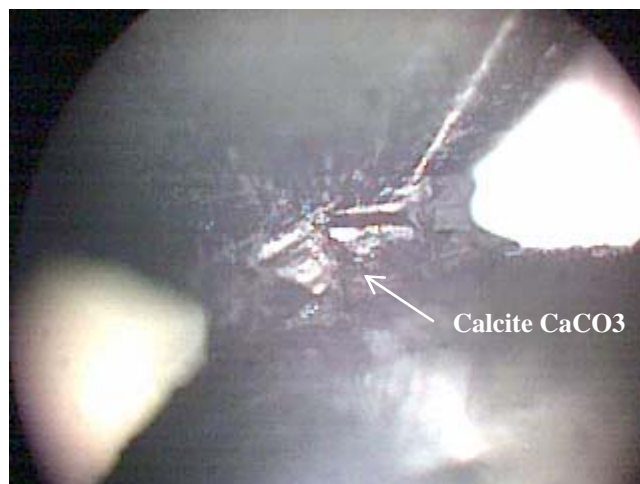
Figure 1 – Cemented basalt crystals (x1000)
