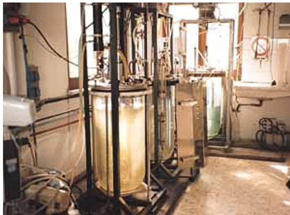
Figure 4 – 100 litre bacterial fermentors
