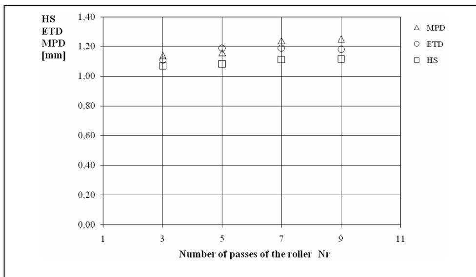
Figure 3 HS, MPD and  $ETD_{iso}$  as function of the number of passes of the roller, Nr
