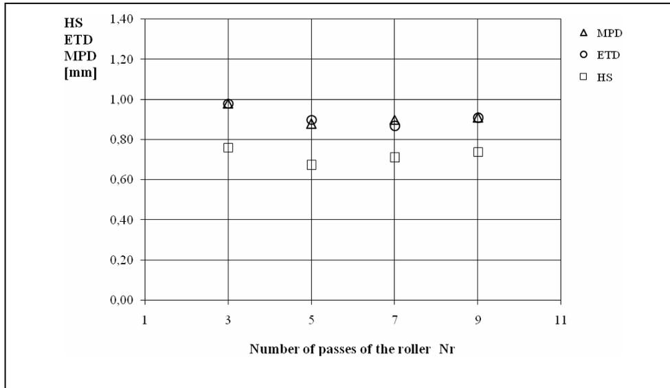
**Figure 4 HS, MPD and ETD<sub>iso</sub> as function of the number of passes of the roller, Nr
