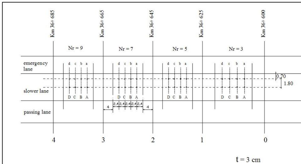
**Figure 2 Representation of the testing site. Layer thickness  $t = 3$  cm**
