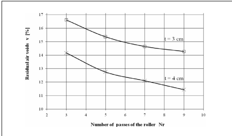
**Figure 10 Residual air voids as a function of the number of passes of the roller, for each layer thickness**
