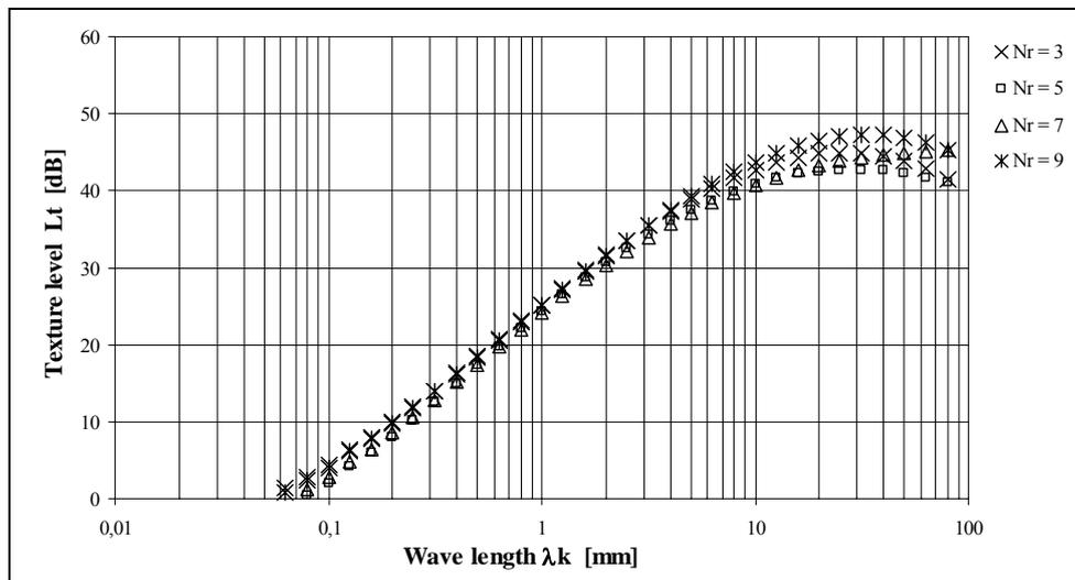
**Figure 8 Texture level - Layer thickness  $t = 4$  cm**
