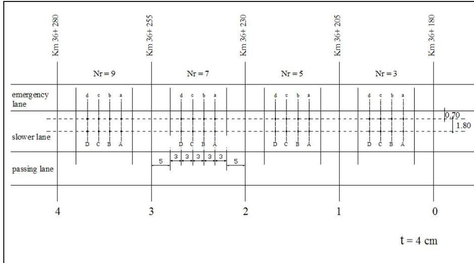
**Figure 1 Representation of the testing site. Layer thickness  $t = 4$  cm**
