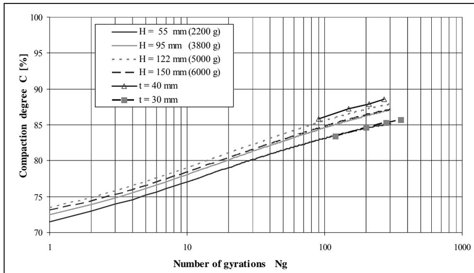
**Figure 11 Comparison between the in situ densification curves and those obtained at the gyratory with specimens of different final height**
