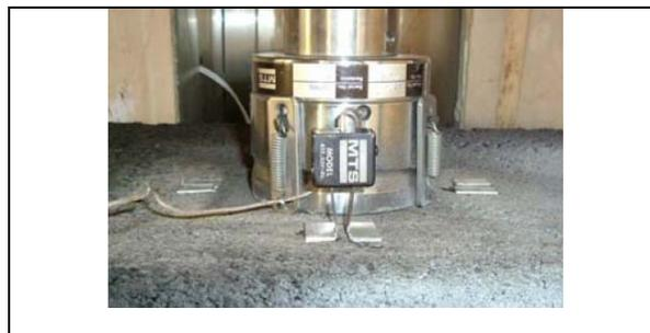
**Figure 5 Extensimeter applied around the load mark**
