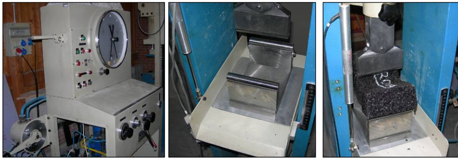
Figure 3 Apparatus for the flexural tests and failure of a specimen
