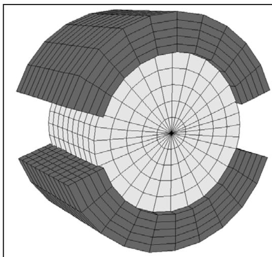
**Figure 1: Marshall Test: Numerical Specimen**
