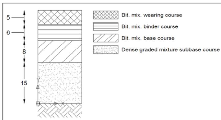
Figure 4: Pavement Layer Scheme, Dimensions In cm
