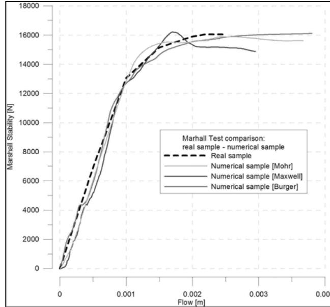
Figure 2: Marshall Test Results Comparison
