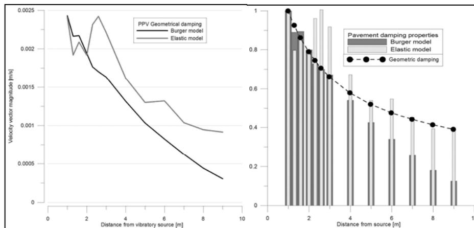
**Figure 8: PPV Geometrical Damping And Damping Properties**
