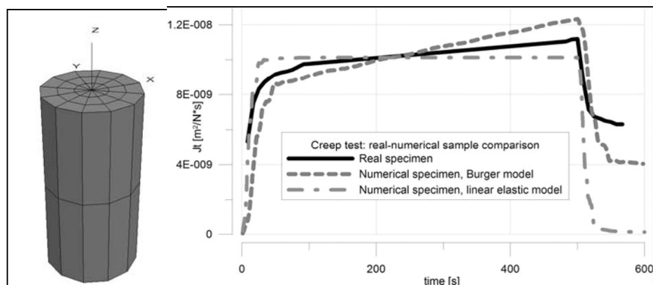
Figure 3: Creep Test, Sample and Results Comparison
