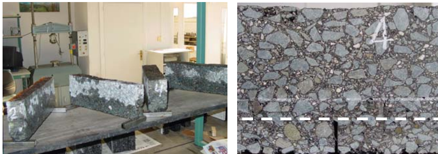
Figure 9 Sample reinforced with Hycore® at the end of the test, 278.000 cycles. No cracks or damage were observed inside of the asphalt concrete overlay.
