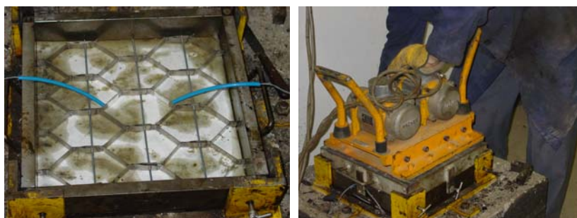
Figure 3 Details of the test sample preparation.
