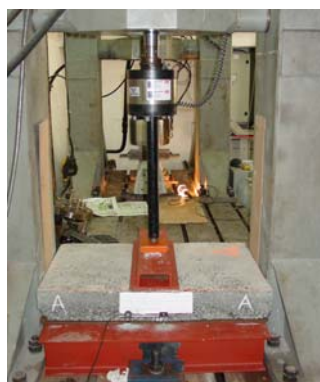
Figure 8 View of the Instron dynamic test machine used to load application in the RCT.
