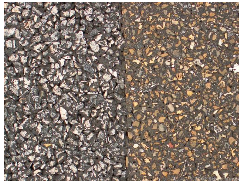
SMA's at the NCAT test track
