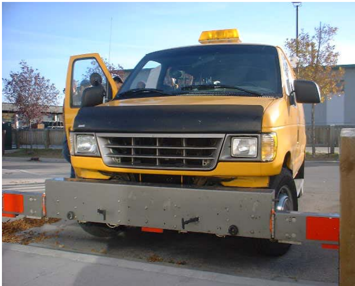
Photograph 1- The automated road surface profiler (ARSP)
