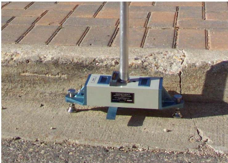
Photograph 2- The Dipstick used for manual profile measurement
