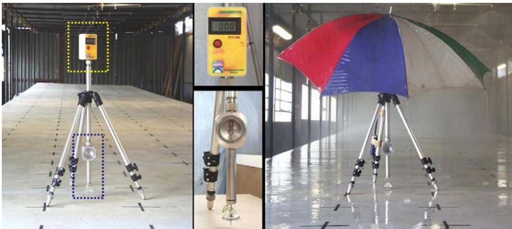
Figure 24 –Limnimeter in running during the simulated rain.
