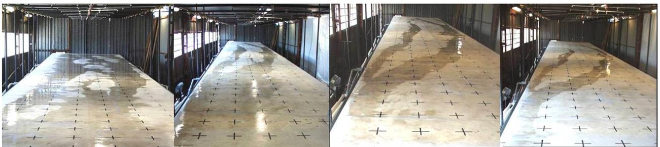
Figure 22 – Temporal sequence of images during the phase of drying on surface 0.
