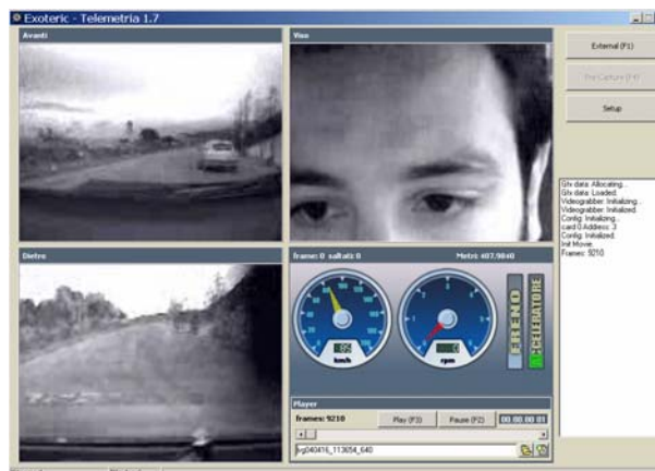
Figure 2: Graphic interface of the three video cameras and the telemetry in real time.
