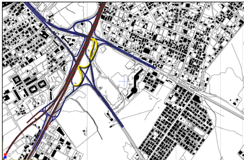
Figure 24 – Present network with the ramps to eliminate
