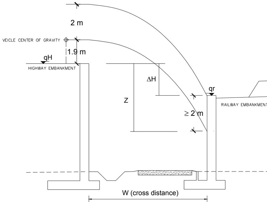
Figure 3: schematisation of the runoff situation in the close sections configuration (ballistic problem)
