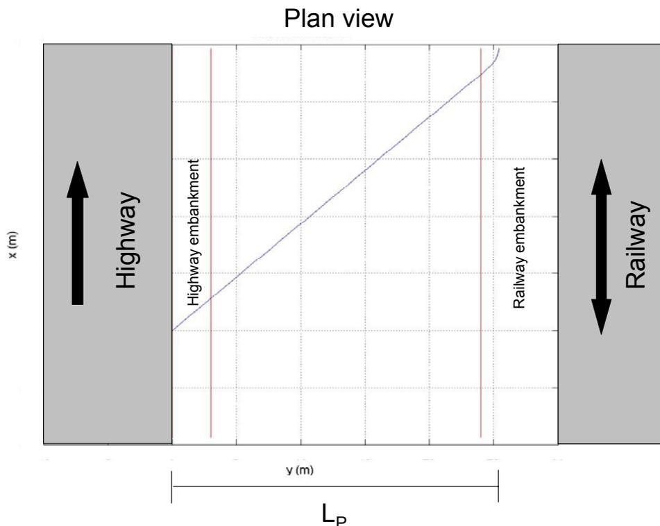
Figure 9: example of plan view of the runoff trajectory
