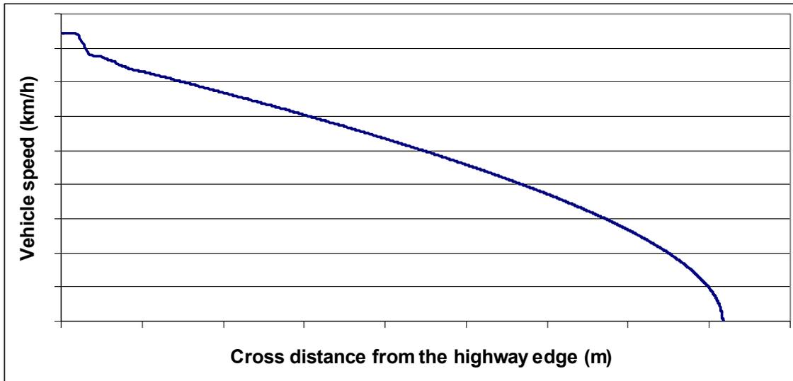
Figure 10: example of speed Vs cross distance diagram
