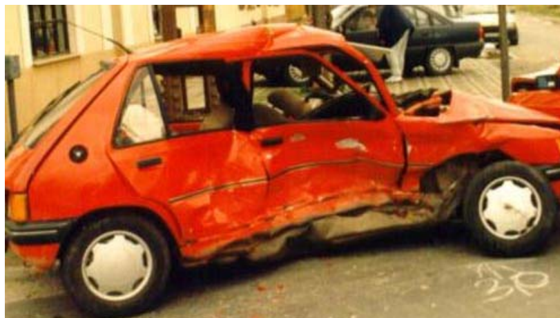
Figure 7 Second vehicle damage (Peugeot 205 1.6).
