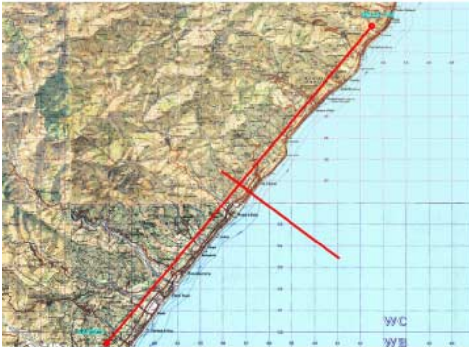
Figure 2: The Thiessen method applied between the stations of Messina and Savoca
