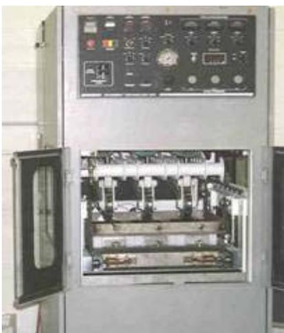
**Photograph 1: Asphalt Pavement Analyzer (APA) in operation**
