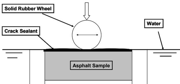
**Figure 7: APA Crack Sealant Bonding Test**
