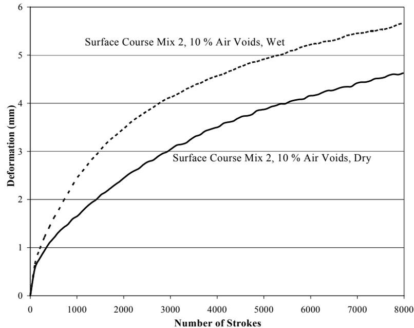
**Figure 5: Permanent deformation of Surface Course Mix 2 tested dry and conditioned in water**
