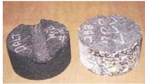
**Photograph 6: The laboratory prepared cylindrical sample on the left developed a deep rut during APA testing. This mix is considered to have poor resistance to rutting. The field core on the right has good resistance to rutting**
