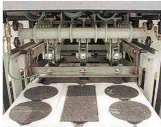
**Photograph 4: One beam and four cylindrical specimens made in the AVC, positioned and ready for testing in the APA**
