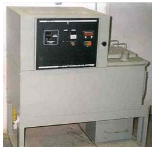
**Photograph 2: A single pugmill Asphalt Laboratory Mixer (ALM) is capable of producing up to 16 kg of an asphalt mix in a single batch**
