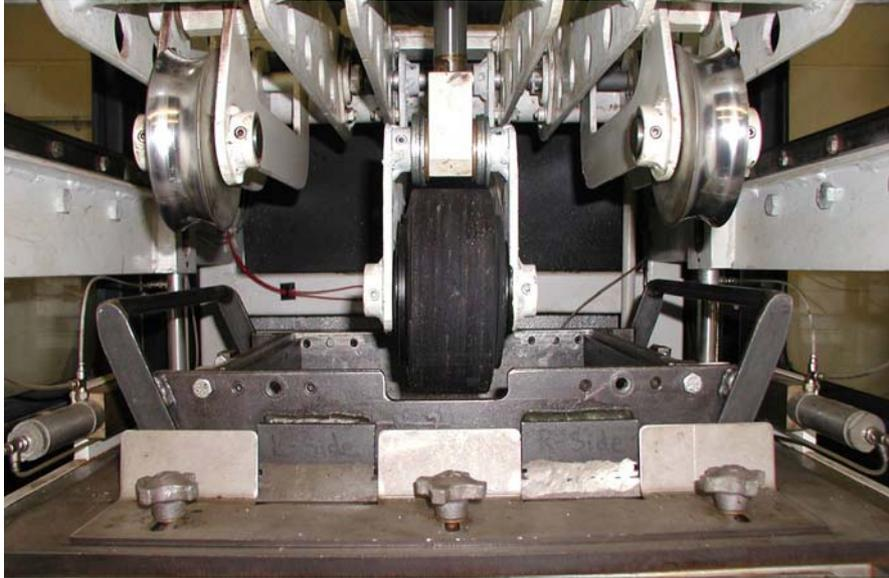
**Photograph 10: APA interface shear resistance and 'large slab' resistance to rutting tests equipment (70 mm wide solid rubber wheel, slab 300 mm x 300 mm)**
