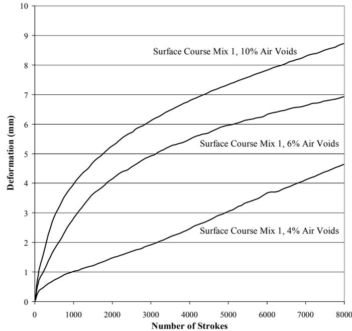
Figure 3: Permanent deformation of Surface Course Mix 1 at 4, 6 and 10 percent air voids
