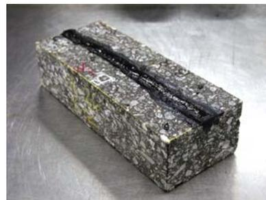
**Photograph 9: A sample of asphalt concrete with routed reservoir filled with crack sealing material**
