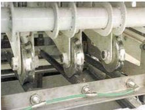
**Photograph 7: Load application system used in the rutting resistance test in the APA**
