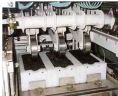
**Photograph 8: Fatigue endurance test setup in the APA. Solid steel wheels are used in the test**
