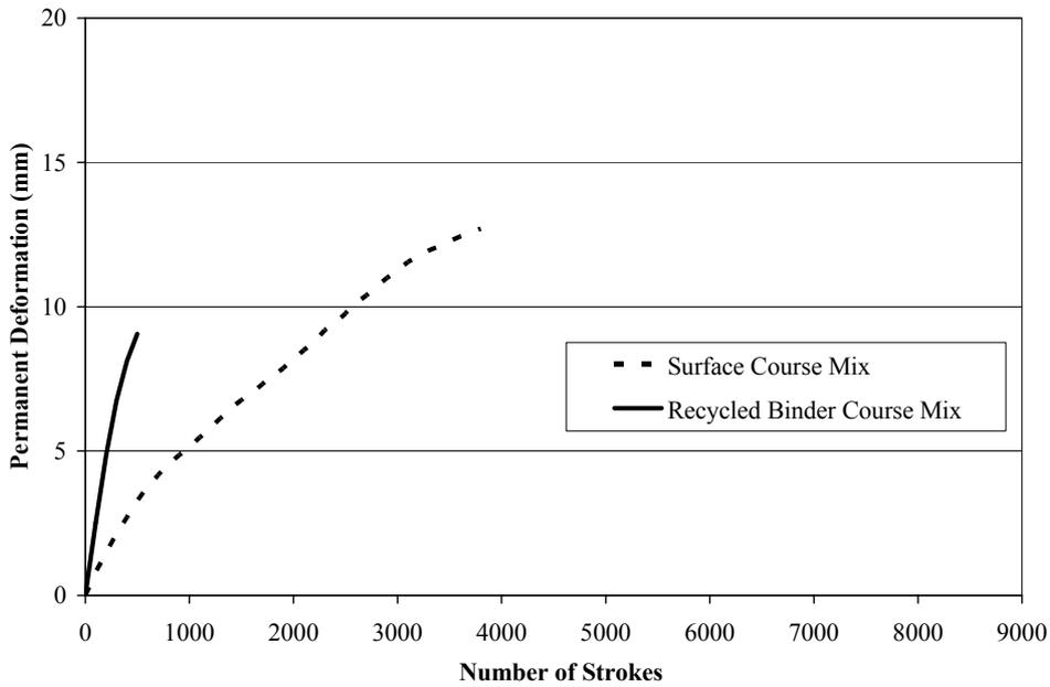
**Figure 2: Permanent deformation of surface course and binder course asphalt concrete in the APA rutting resistance test**
