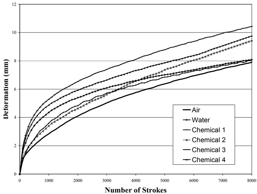
**Figure 6: Permanent deformation of asphalt concrete samples conditioned in four different chemical solutions and water**
