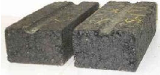
**Photograph 5: Beam samples used for APA rutting resistance testing. The mix on the left developed a deep rut during testing and is considered to have poor resistance to rutting. The mix on the right has good resistance to rutting**
