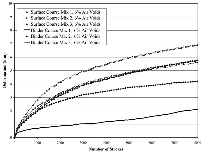
Figure 4: Permanent deformation of binder and surface course asphalt mixes incorporating different types of aggregate
