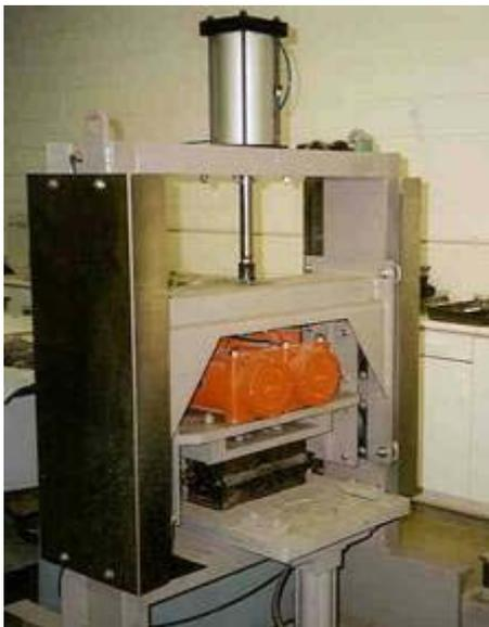
**Photograph 3: Asphalt Vibratory Compactor (AVC) in operation**
