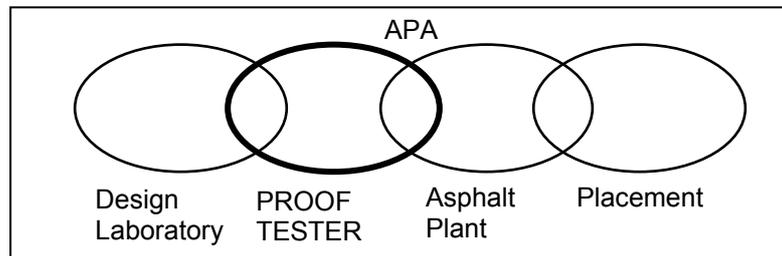
**Figure 1: The Asphalt Pavement Analyzer is considered to provide the missing link between laboratory testing and potential field performance of asphalt mixes**
