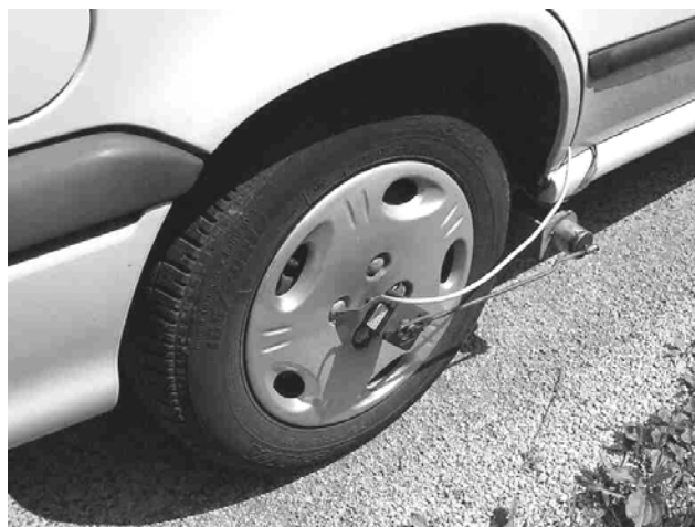
Figure 2. Position of the angular-variable differential transformer
