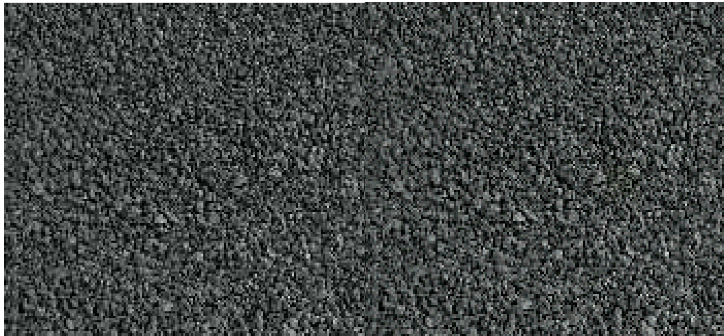
Figure 8: Mix 3 showed the best superficial aspect and compactness
