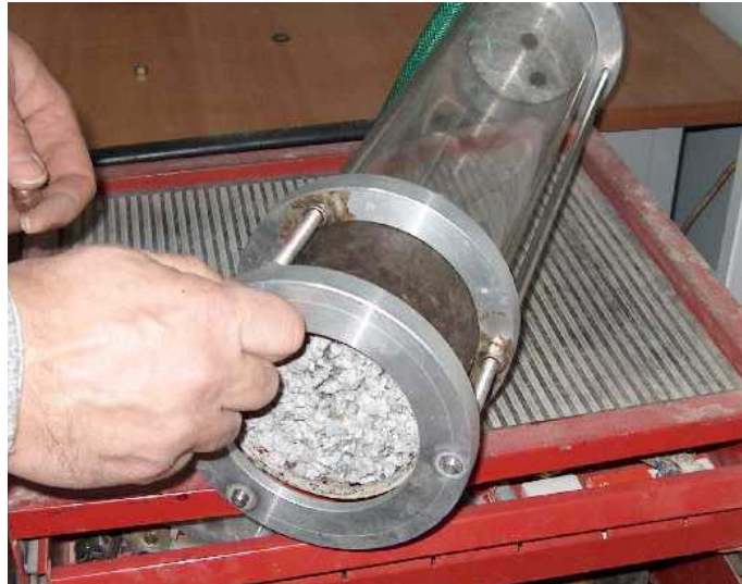
Figure 14: Water column permeameter for the permeability assessment
