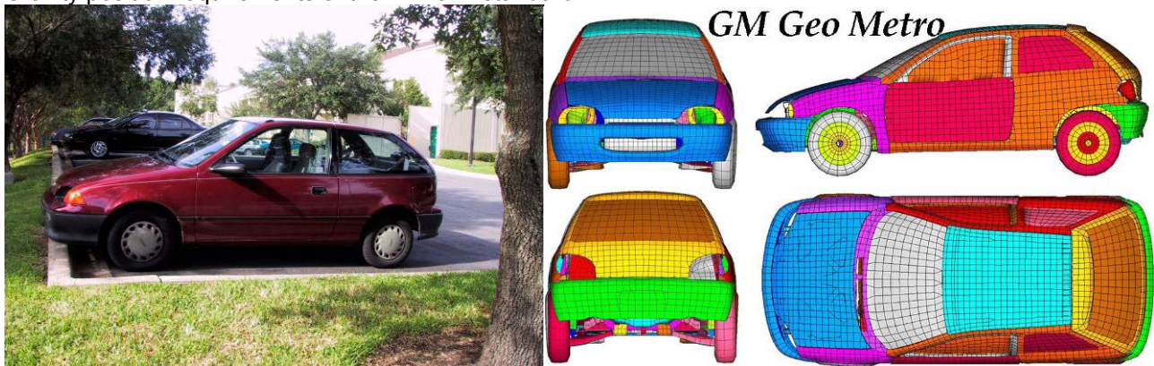
Figure 12 – Lightweight vehicle used for the TB11 test (GM Geo Metro) – National Crash Analysis Center
