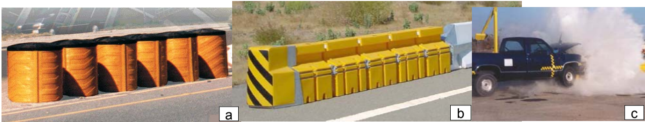
Figure 7: a) Sand barrels, b) inertial end treatment, c) full scale impact test on inertial end treatment
