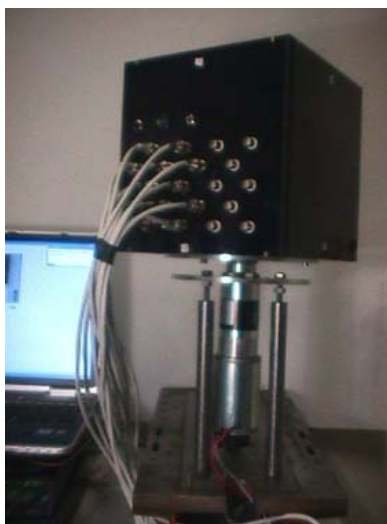
Fig. 10: Dynamic calibration set up: blue-box mounted on a rotating platform close loop controlled
