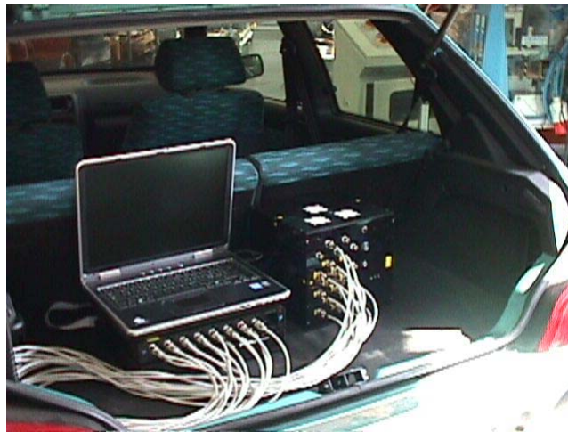
Fig. 2: The blue-box system set up for the test on the road
