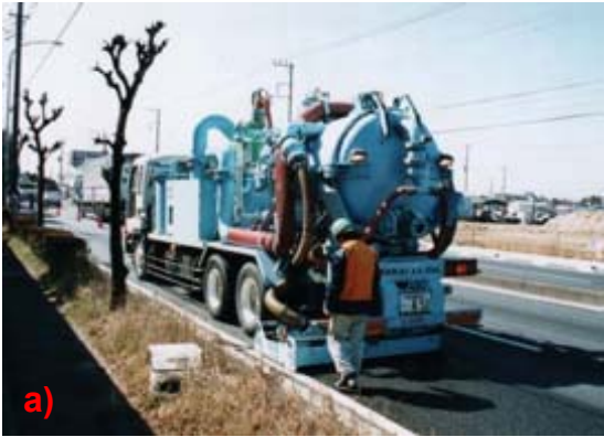
Figure 5a, b: View of a cleaning machine (a) with a detail of the cleaning device (b) (Sakai, 2004).
