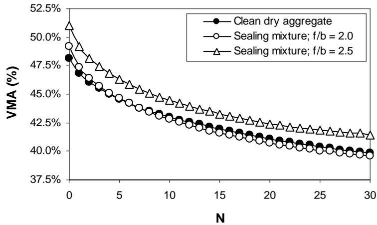
**Figure 4 - Compaction curves of the aggregate and of the design mixtures**
