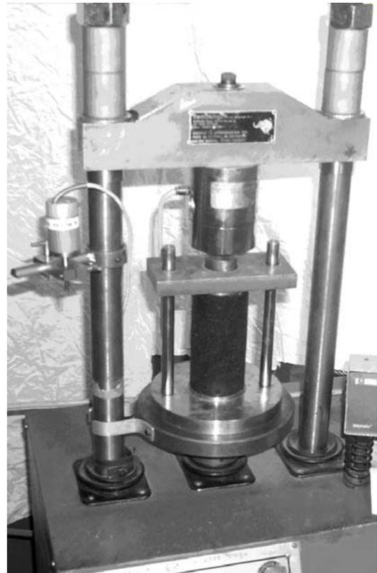
**Figure 5 – Simple compression test equipment and results**
