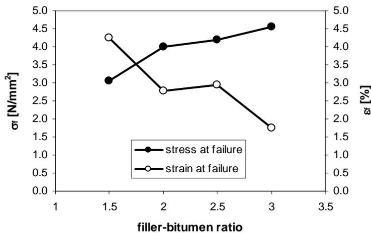
**Figure 2: Direct tension test results obtained at -6°C**
