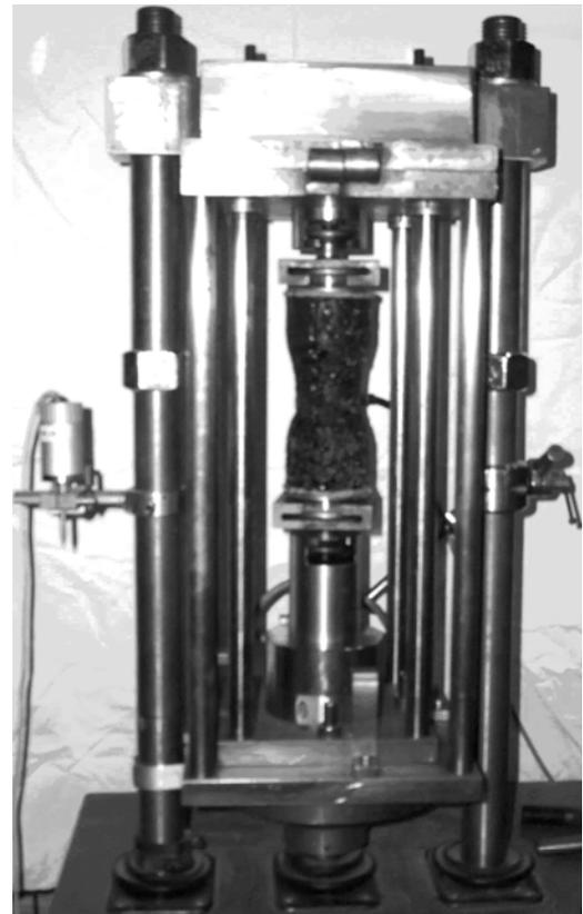
Figure 6 – Direct tension test equipment and results
