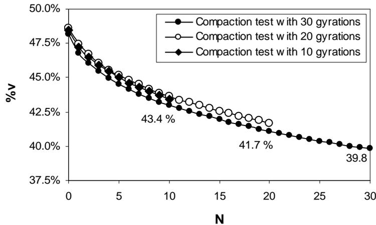
**Figure 3 – Compaction curves of the single-sized aggregate**
